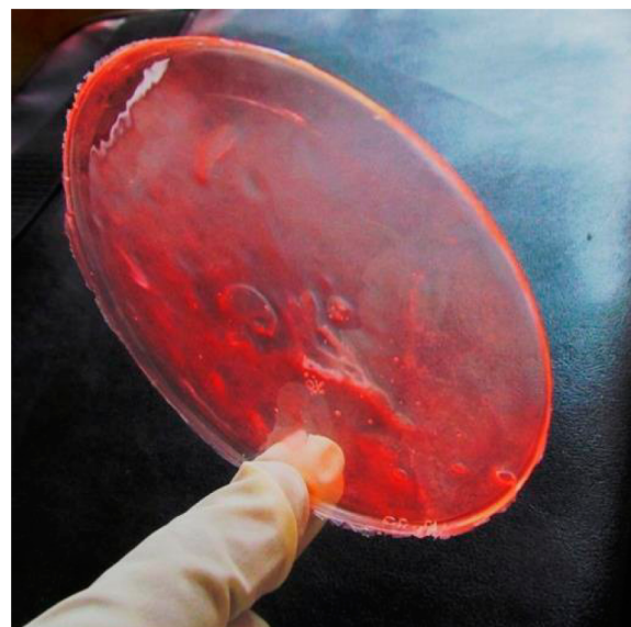
Figure 11. Photograph of a PMMA film doped with 4 wt % of (\text{NBu}_4[\text{EuL}])_2 under natural daylight.
